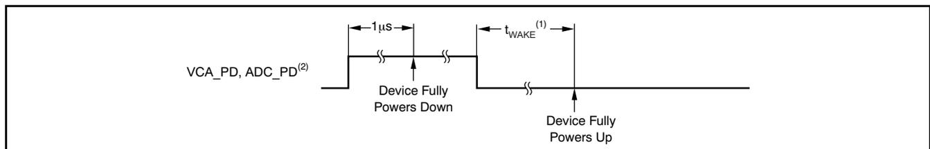
Power-up time shown is based on  $1\mu\text{F}$  bypass capacitors on the reference pins.  $t_{\text{WAKE}}$  is the time it takes for the device to wake up completely from power-down mode. The AFE5805 has two power-down modes: complete power-down mode and partial power-down mode.
