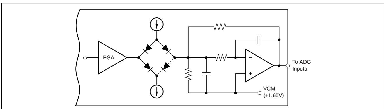
Figure 49. Clamping Stage and Low-Pass Filter (Simplified Schematic)
