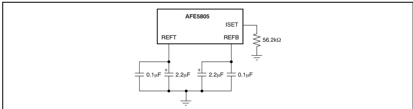
**Figure 58. Suggested Decoupling on the Reference Pins**
