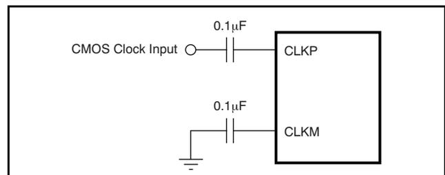
Figure 57. Single-Ended Clock Driving Circuit When  $\text{DIFF\_CLK} = 1$
