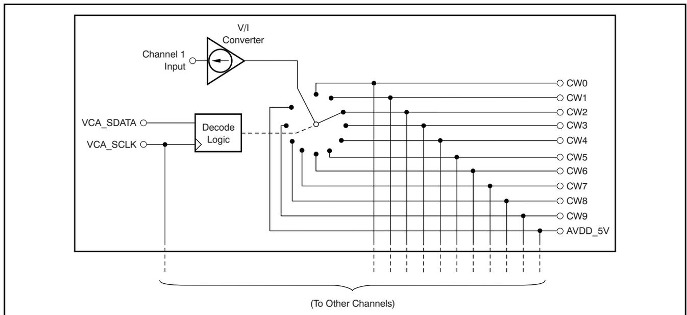
**Figure 42. Basic CW Cross-Point Switch Matrix Configuration**
