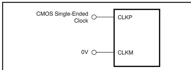
Figure 54. Single-Ended Clock Driving Circuit ( $\text{DIFF\_CLK} = 0$ )
