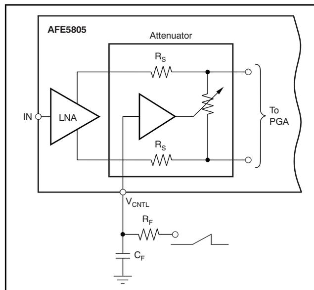
**Figure 52. External Filtering of the  $V_{CNTL}$  Input**
