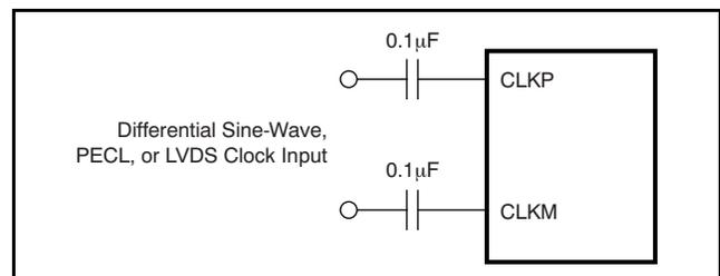
Figure 56. Differential Clock Driving Circuit ( $\text{DIFF\_CLK} = 1$ )
