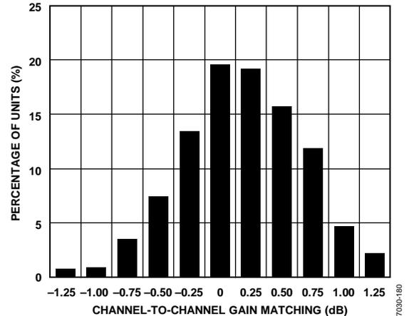
Figure 10. Gain Match Histogram, GAIN+ = 0.3 V
