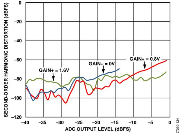
Figure 21. Second-Order Harmonic Distortion vs. ADC Output Level
