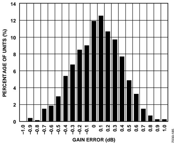
Figure 8. Gain Error Histogram, GAIN+ = 0.8 V
