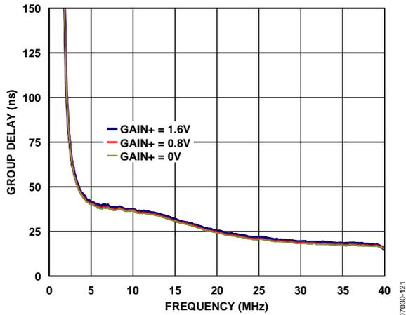
Figure 18. Antialiasing Filter (AAF) Group Delay Response
