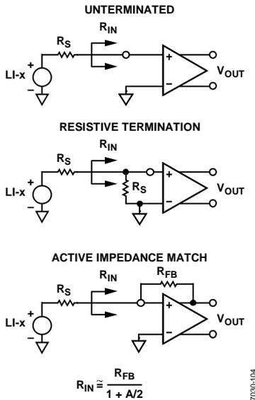
Figure 41. Input Configurations
