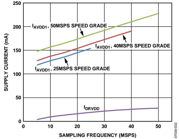
Figure 61. Supply Current vs.  $f_{SAMPLE}$  for  $f_{IN} = 5$  MHz
