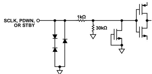
Figure 30. Equivalent SCLK, PDWN, or STBY Input Circuit
