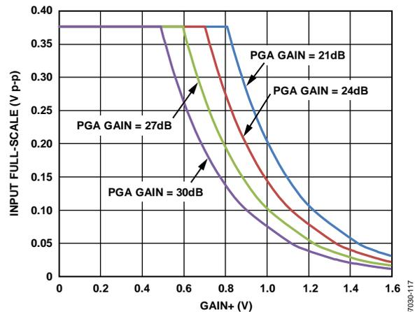
Figure 48. LNA with 15.6 dB Gain Setting/VGA Full-Scale Limitations
