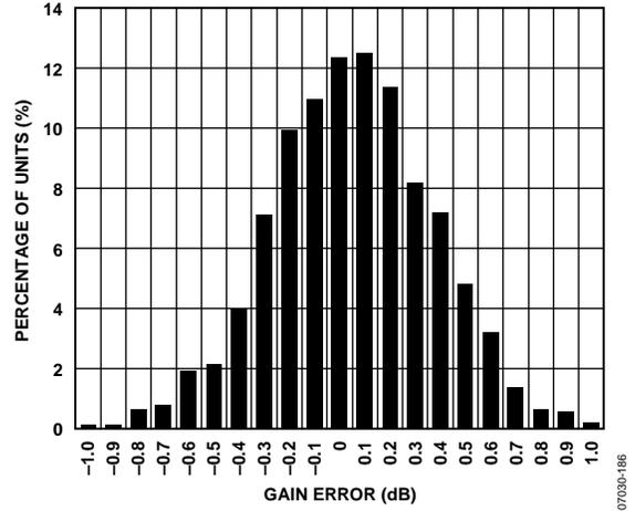
Figure 9. Gain Error Histogram, GAIN+ = 1.44 V
