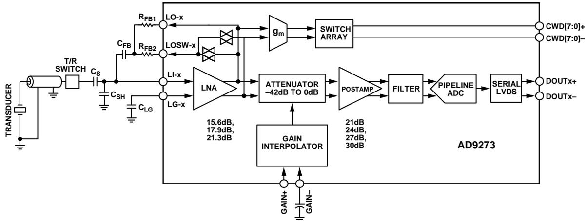
Figure 38. Simplified Block Diagram of a Single Channel
