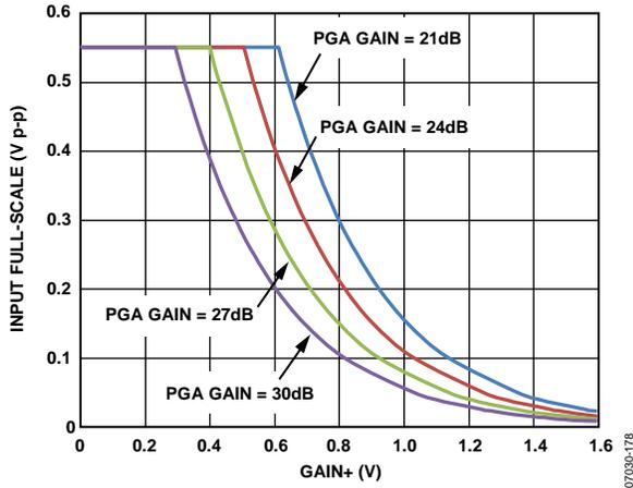
Figure 49. LNA with 17.9 dB Gain Setting/VGA Full-Scale Limitations
