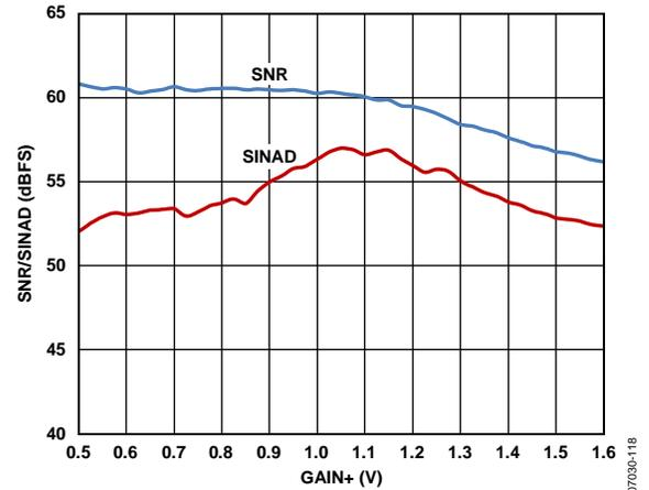
Figure 16. SNR/SINAD vs. GAIN+, AIN = -1.0 dBFS
