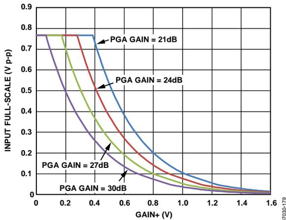
Figure 50. LNA with 21.3 dB Gain Setting/VGA Full-Scale Limitations
