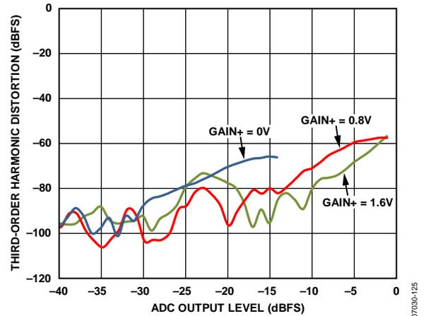
Figure 22. Third-Order Harmonic Distortion vs. ADC Output Level
