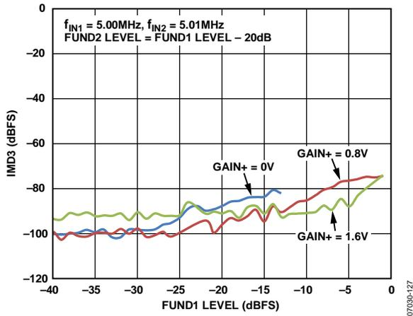
Figure 24. IMD3 vs. Fundamental 1 Amplitude (FUND1) Level
