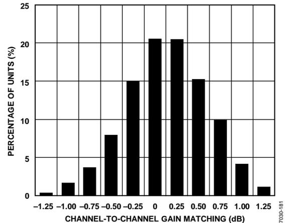
Figure 11. Gain Match Histogram, GAIN+ = 1.3 V
