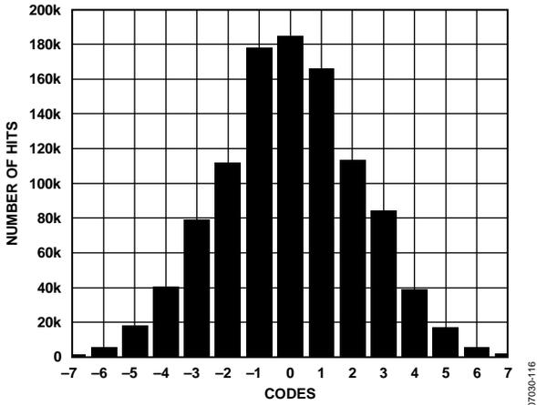
Figure 13. Output-Referred Noise Histogram, GAIN+ = 1.6 V
