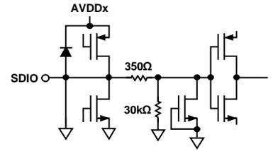
Figure 28. Equivalent SDIO Input Circuit
