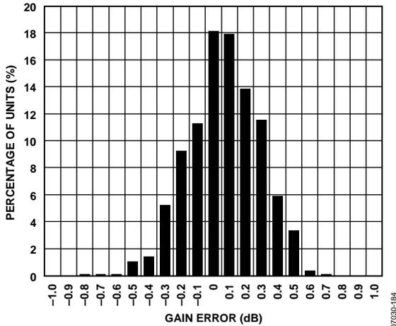
Figure 7. Gain Error Histogram, GAIN+ = 0.16 V
