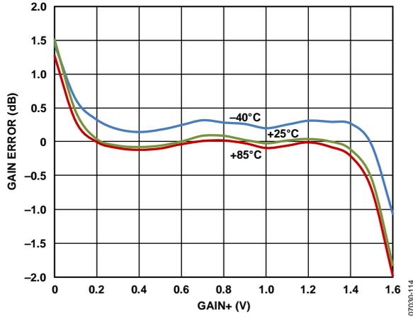
Figure 6. Gain Error vs. GAIN+ at Three Temperatures
