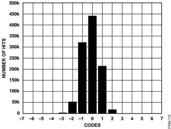
Figure 12. Output-Referred Noise Histogram, GAIN+ = 0.0 V
